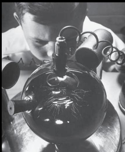
Wilson cloud chamber tracing the path of alpha particles through water-alcohol vapour.
